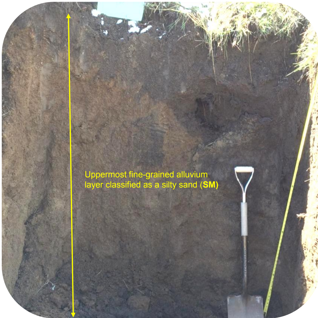
Photo # 9: Test Pit TP-2 Trench Sidewall Showing Geologic Soil Profile
