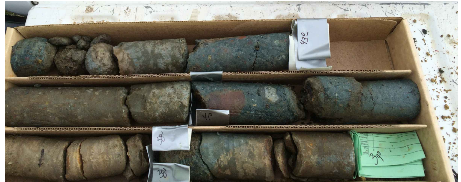
PHOTO #4: CORE DEPTH 36'-43' , BASALTIC LAHAR BEDROCK
