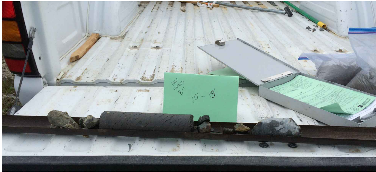
PHOTO #1: CORE DEPTH 10'-13' , NOTE BASALT BOULDER IN SAMPLE, GLACIAL OUTWASH
