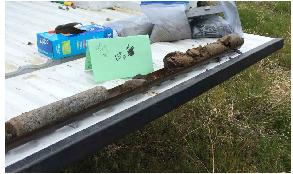
PHOTO #2: CORE DEPTH 13'-18' , NOTE GRANITIC BOULDER VISIBLE IN SAMPLE, GLACIAL OUTWASH
