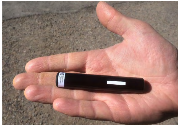
An acoustic tracking device like the one shown is implanted in Lahontan cutthroat trout to track their migration from Pyramid Lake into the Truckee River. Credit: Erik Horgen/USFWS
