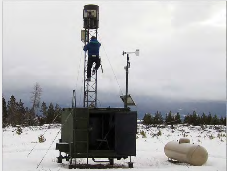
A cloud seeding generator near the Winter Park ski area in Colorado | Photo: Desert Research Institute (DRI)
