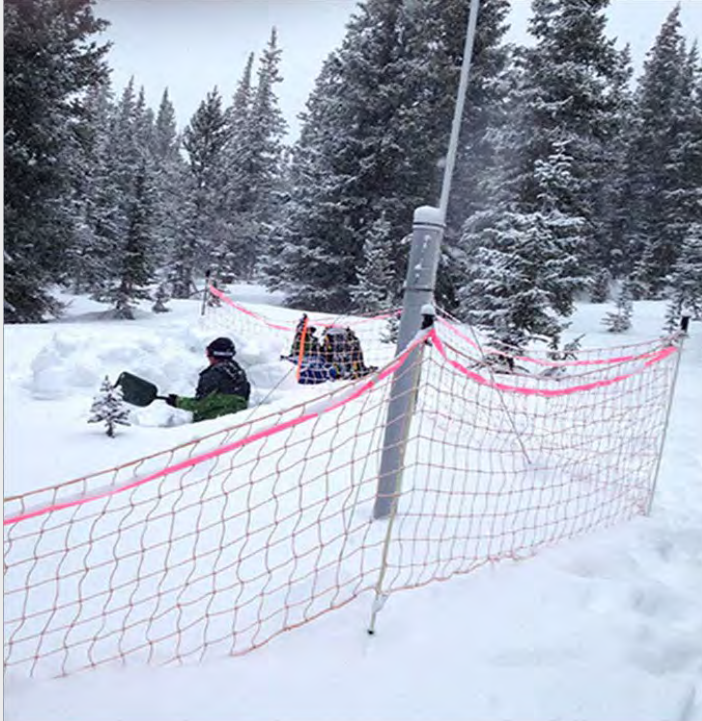
Snow pit at Winter Park ski area to sample for silver iodide | Photo: Desert Research Institute (DRI)
