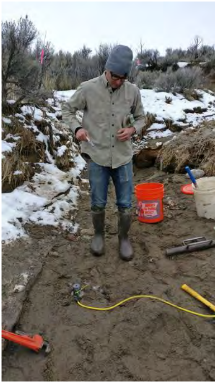
Installation of a temperature probe (TROD) in Bird Springs drainage. (Public domain.)
