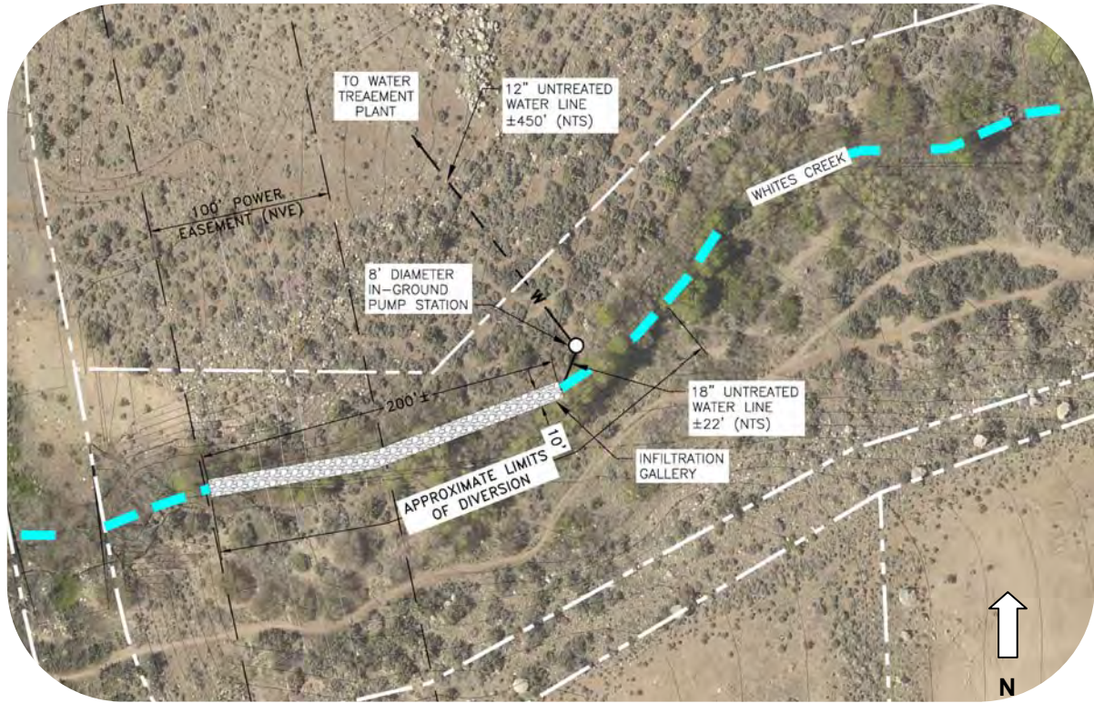
Figure 3: Tentative Site Layout-Diversion Feature #1 3 N.T.S
