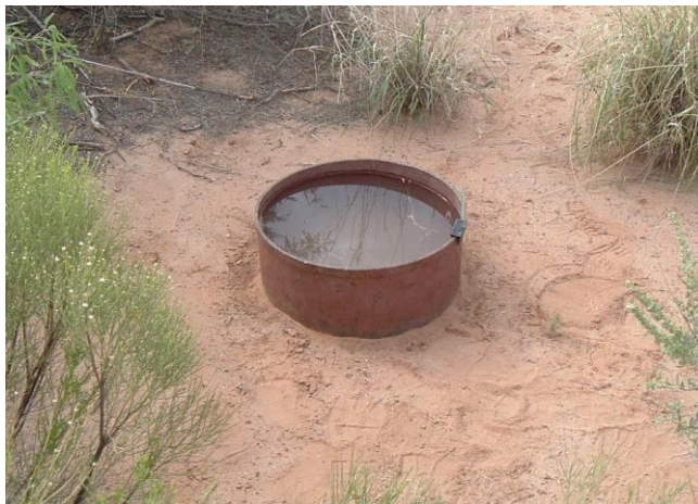
Figure 1a. Cylinder infiltrometer testing
