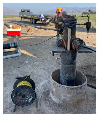
Aquifer Pumping Test Set-Up
