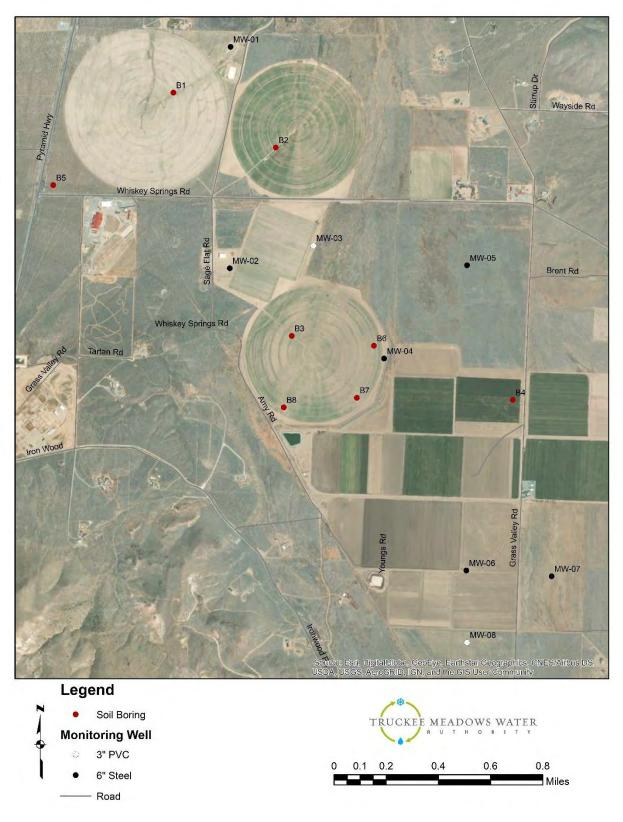
Figure 4. Soil borings and monitoring wells constructed for this project.
