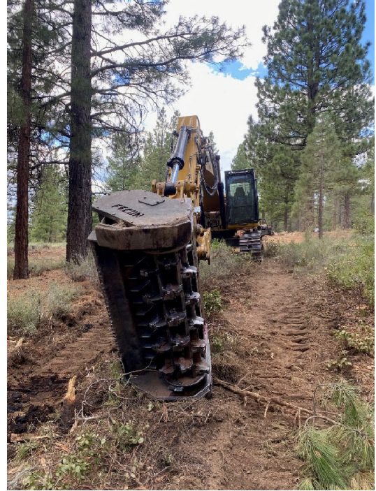
A masticator at the Ladybug Project in 2023 used to grind trees up to 16" in diameter
