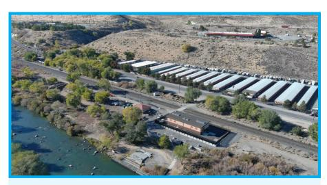
The Orr Ditch Booster Pump Station is a backup raw water source for Chalk Bluff Water Treatment Plant. If the Highland Canal (the main raw water source) needs to be taken offline, the Orr Ditch Pump Station comes online to convey water to Chalk Bluff.
