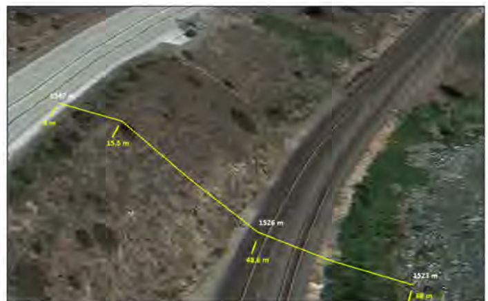
This screen capture from Google Earth (with elevation and distance added) shows the close spatial proximity of Interstate 80 (I-80), the rail route, and the Truckee River at 12 km upstream from the first Truckee Meadows Water Authority water treatment plant. Elevation (shown in white) drops by 21 m from the right edge of the I-80 pavement to the left edge of the rail line ballast. The total distance (shown in yellow) from the right edge of the I-80 pavement to the bank of the Truckee River is approximately 86 m.
