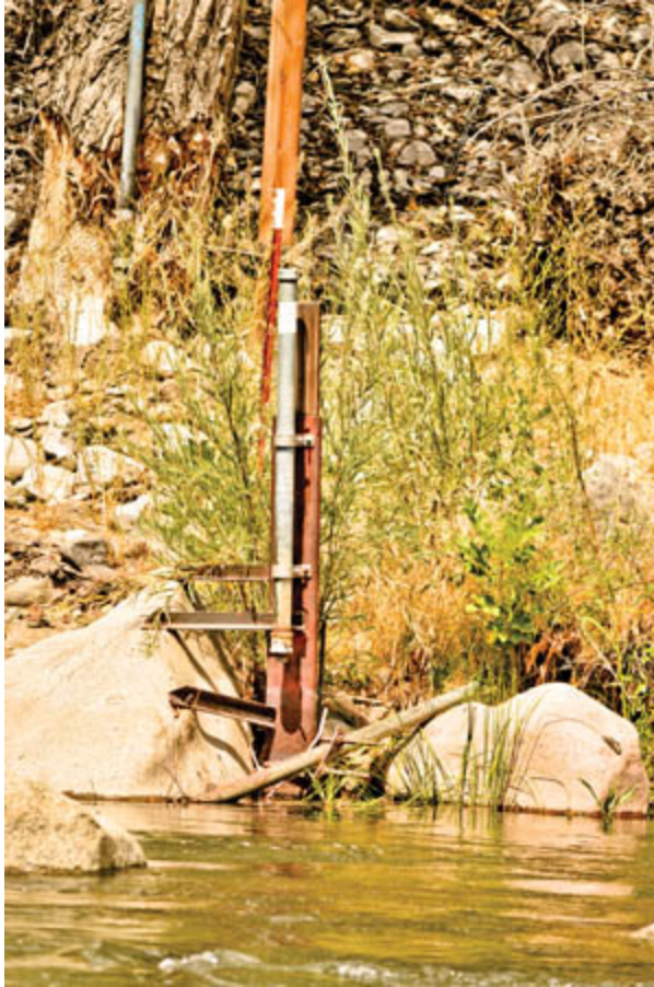
A depth gauge on the Truckee near Sutro Street is one of several in the valley that keep water officials informed. PHOTO/JERI CHADWELL-SINGLEY
